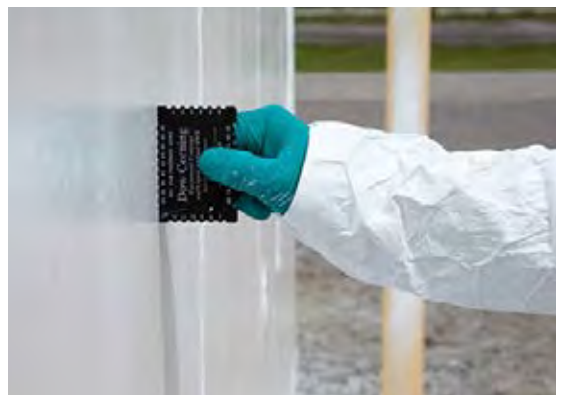
Demonstrating usage of wet mil gauge
