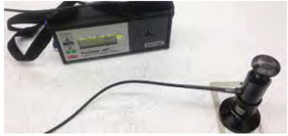
Figure 12. Adhesion Test Using ASTM D4541
