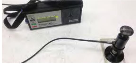
**Figure 12. Adhesion Test Using ASTM D4541**
