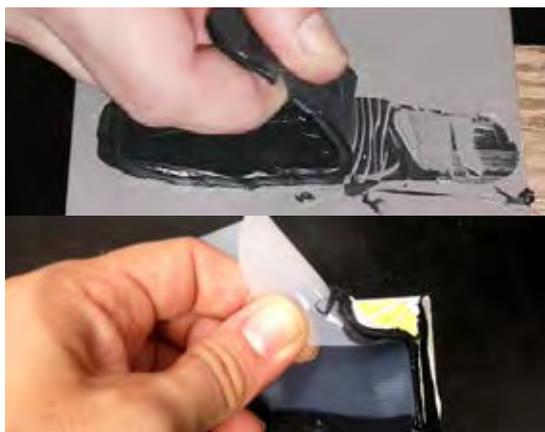
Figure 3: Tab Adhesion Test Procedure
