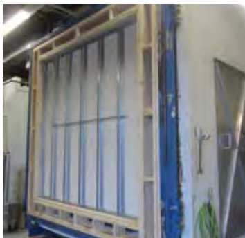
Wall tested for air, water and structural performance
