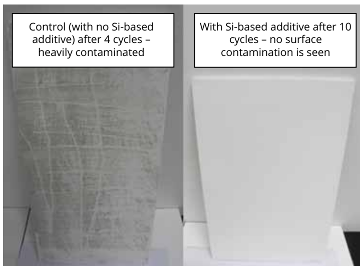
FIGURE 3 » Surface of architectural paint – with and without a Si-based additive – after brushing with standard synthetic dirt paste and washing.
