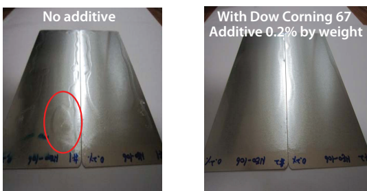
FIGURE 4 | Surface appearance of a waterborne polyurethane acrylic wood parquet lacquer with and without Dow Corning 67 Additive (added at 0.2% by weight in the total formulation).
